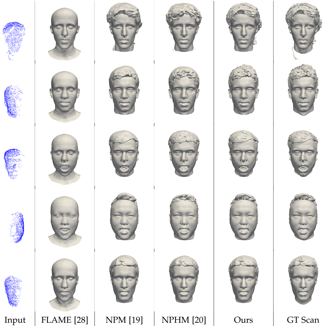
Figure 6.1: Identity fitting comparison. At inference time we fit partial point clouds obtained from single view depth maps to reconstruct full head geometry. We compare our method to widely-used state-of-the-art parametric head models including FLAME [28], NPM [19] and NPHM [20]. Our proposed approach is able to capture more high frequency surface details especially in the hair regions.
